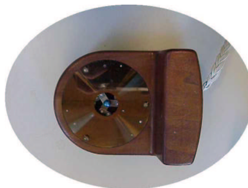
Figure 1. The Penbased Haptic Display[1] was used for these experiments. It supports planar motion within 1.5x1.5cm 2 workspace. Peak force is 1.4N and friction level is less than 10nN and resolution is higher than 0.02mm.
