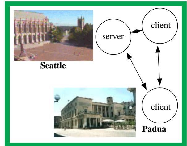
A TCP-IP based communication software module allows multiple remote players to interact. Extremely low latency and high collision detection sampling rate are needed to provide realistic force feedback.
