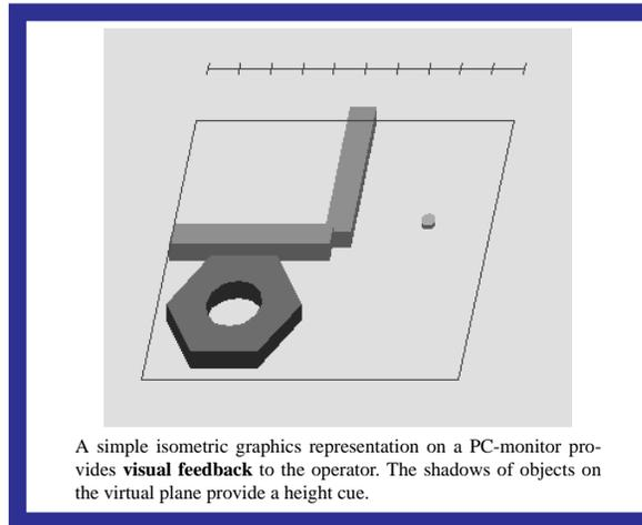
A simple isometric graphics representation on a PC-monitor provides **visual feedback** to the operator. The shadows of objects on the virtual plane provide a height cue.
