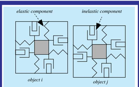
Virtual objects are modeled as mechanical impedances (mass, stiffness and damping). The interaction forces and the objects motions are computed using **collision detection** and **dynamics** software modules [1]. The stiffness components model elastic collisions while dampers dissipate energy.
